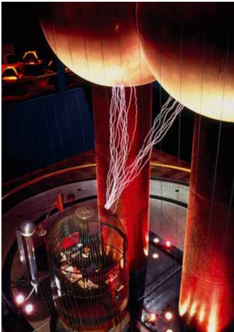
Figure 4.10 Faraday Cage with Van de Graaf generator. Boston Museum of Science, USA. Photo: Peter Menzel/Science Photo Library. Faraday showed that electrical disturbances always remain on the outside of a closed, conducting surface, such as a cage made of copper wire mesh. In this picture the operator controlling the electrical machine from inside the cage is quite safe from the large sparks hitting the cage (the dome-shaped structure at the bottom of the picture). For the same reason, passengers in aeroplanes are safe during lightning strikes, and mobile phones do not work in lifts.
